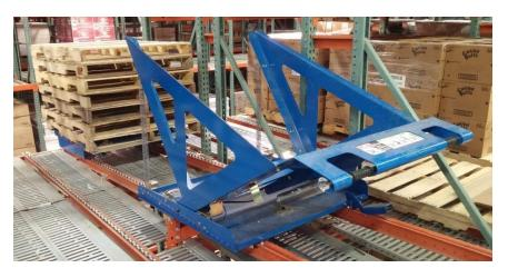
A customer of Automation Plus, a Division of CSF Incorporated in Stoughton, WI came to them with a problem. They needed a solution for stacking empty pallets in their full case picking modules that was both ergonomic for the picker and more efficient for the fork truck driver.
